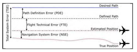
Each aircraft operating in RNP airspace must have Total System Error components in the cross- track and along track directions that are less than the RNP value for 95% of the flying time.
