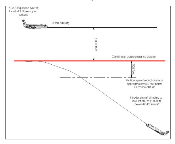
Figure III-3-3-1. Representative HVR Encounter Geometry
